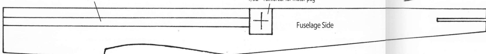
Build the fuselage with the two sides and formers F1 and F2, then add the lower fuselage. Cut here to allow the lower wing to be fitted. Add the cabane strut assembly then finally the curved decking
